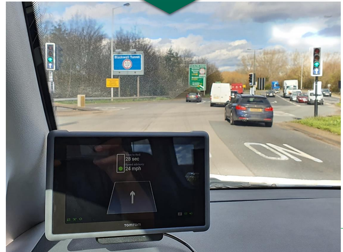
HMI showing GLOSA service displaying live traffic signal information from TfL's Urban Traffic Control system, and providing advice relating to the time to a red signal
