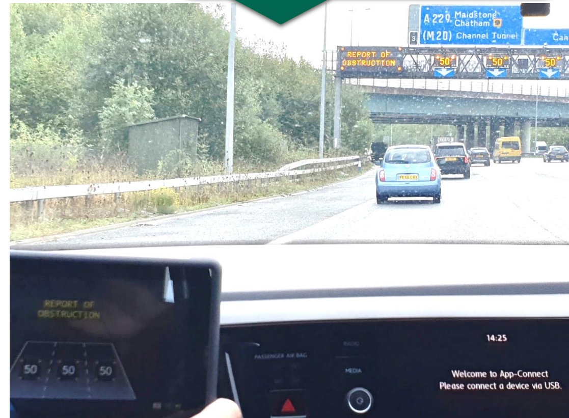
HMI showing In-Vehicle Signage service providing live traffic information from Highways England's NTIS traffic information service, and replicating live VMS signing
